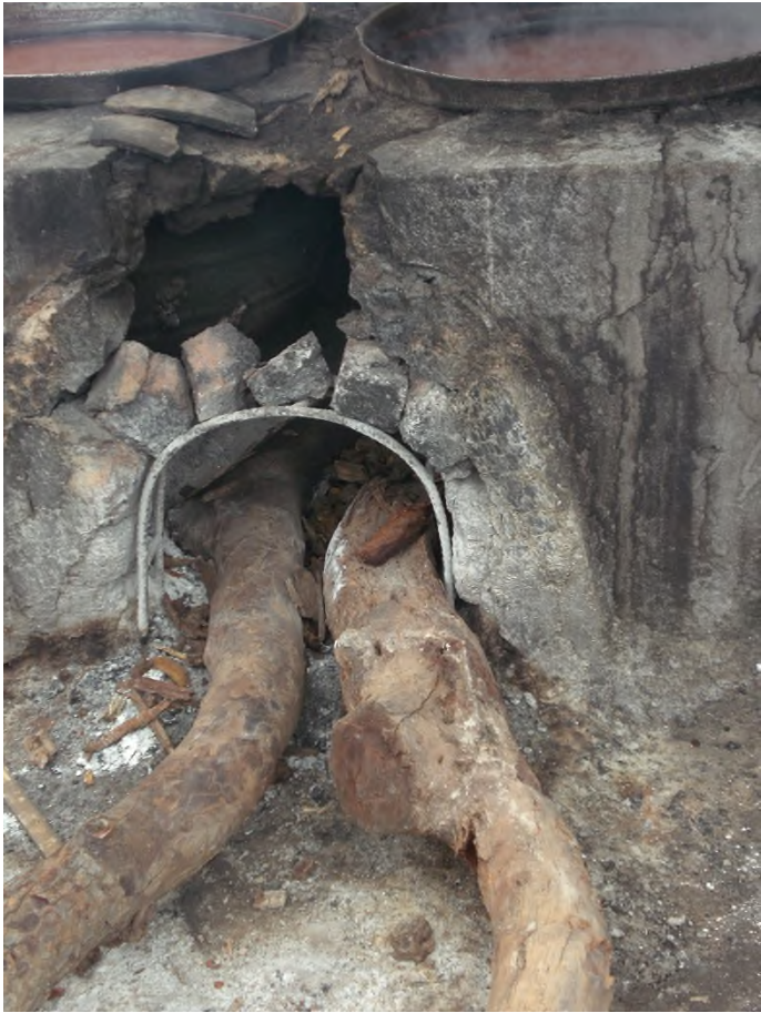
Photo 9: A Roudé stove with a broken door (b)
